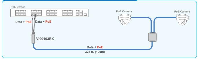
The NetMux™ Vi00103 can connect two cameras at standard UTP distances over a single cable.
