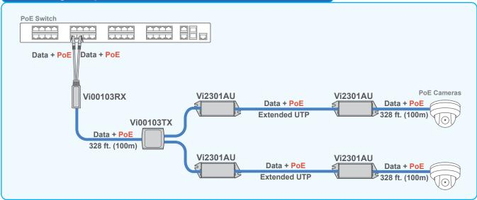
The NetMux™ Vi00103 along with Vi2300 series can connect two cameras at extended UTP distances.
